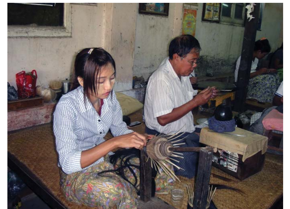
Lacquer worker weaving horsehair onto a frame prior to applying laquer.
